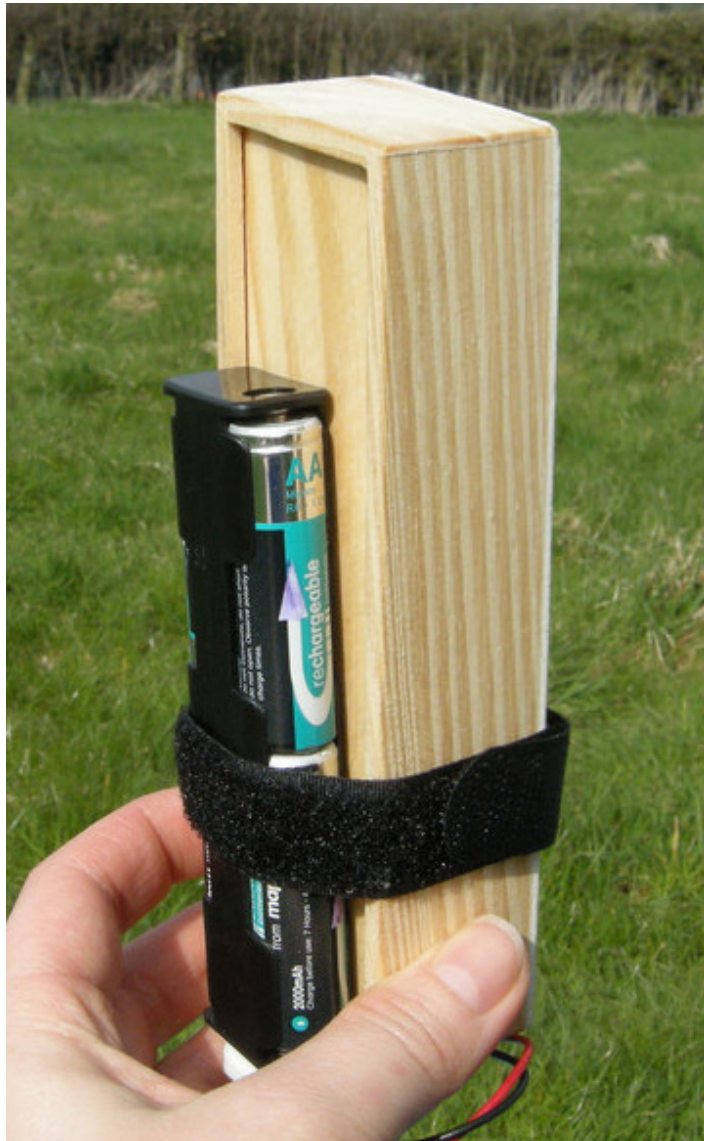
Figure 12. The ‘pocket version’ of the pod. It has the same functionality as the paper versions, but is built into a small wooden box that can safely be carried in a back pocket or the bottom of a rucksack.
